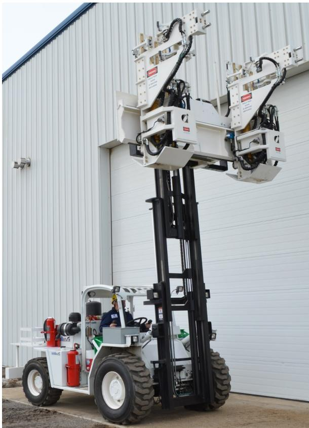
The DynaBolter V4.0 takes the safety features of a DynaBolter and applies it to the production aspect of mining. Designed to improve the process of installing belt and cable runs, the V4.0 has two drill drives, two bolt drives and two 6-bolt carousels. These features come standard but the DynaBolter V4.0 also includes operator focused options like a front-mounted travel camera, lunch kit and water jug holder and an over 30-bolt storage system.
