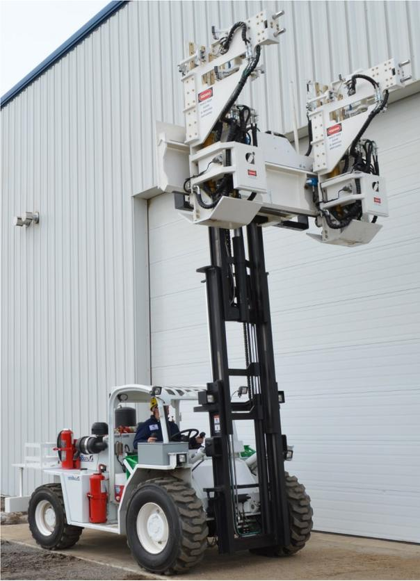
The DynaBolter V4.0 takes the safety features of a DynaBolter and applies it to the production aspect of mining. Designed to improve the process of installing belt and cable runs, the V4.0 has two drill drives, two bolt drives and two 6-bolt carousels. These features come standard but the DynaBolter V4.0 also includes operator focused options like a front-mounted travel camera, lunch kit and water jug holder and an over 30-bolt storage system.
